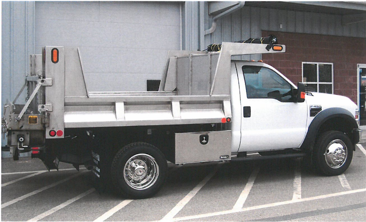
THE PITTSBURGH INDUSTRIAL TRUCK BED - STAINLESS STEEL shown with 13" high sides, optional tarp system and optional salt spreader
